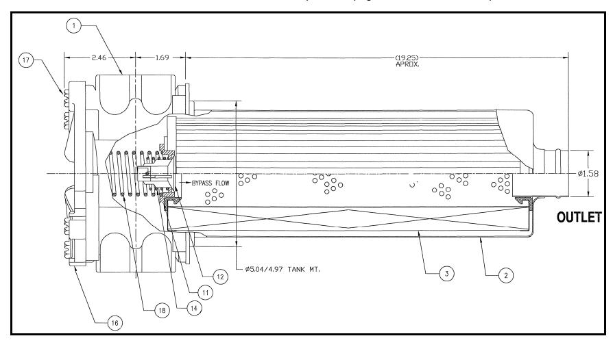
F5D100 In-Tank Filter Assembly – Pg 2 [View of head and of the adaptor for units using HF4-050 elements]
