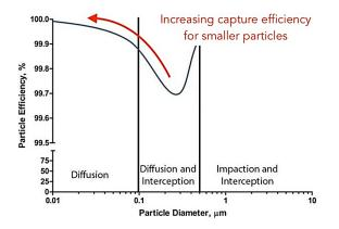
Just a note - HEPA filters are designed to arrest very fine particles effectively, **but they do not filter out Volatile Organic Compounds (VOC's) and odor molecules.** Since gases are not particles, they move and behave differently in the air. To capture VOC's and odors, the HEPA filters would need to be supplemented by other technology such as activated carbon or others.
